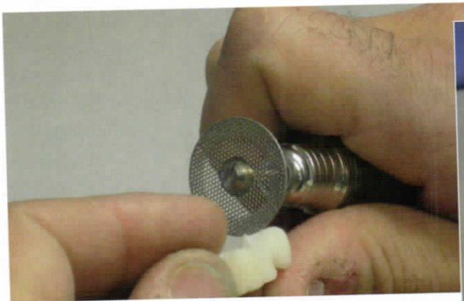
Figure 8: The sprue was cut off the crown restoration after pressing and divesting.
